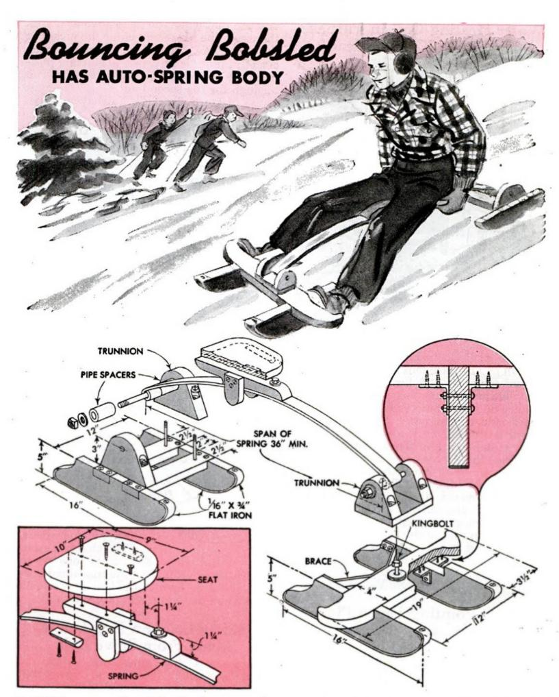
THE bumpier the slide the better with this spring-bodied bobsled, which is steered with the feet so that the rider can hold on to the seat. The main leaf of an auto spring is held by lengths of iron rod set through wooden trunnions, which are bolted to cross members screwed to sled runners shod with strips of flat iron. Since the rear trunnions are widely spaced to prevent the sled from upsetting, the spring is centered on the rear rod by pieces of pipe. On the more closely spaced front
