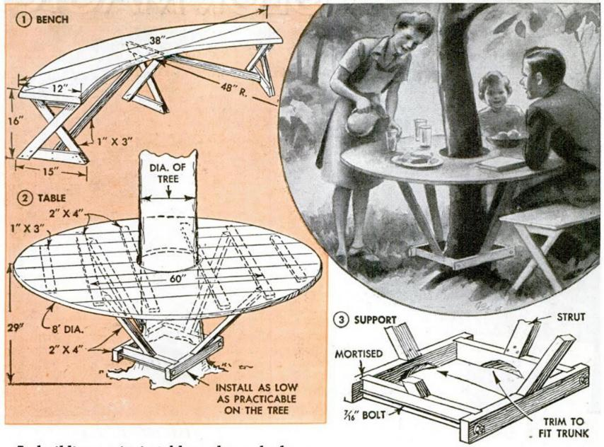
In building a picnic table under a shade tree, it isn't necessary to injure the tree by using lag screws or nails to hold the table in place. Just prop the table top on four struts nailed to a frame, which fits around the tree trunk. The frame is made by mortising four lengths of 2 by 4-in. stock, trimming the inner edges to conform to the shape of the tree trunk near the ground, and then clamping the pieces together tightly with two long bolts as in Fig. 3.
